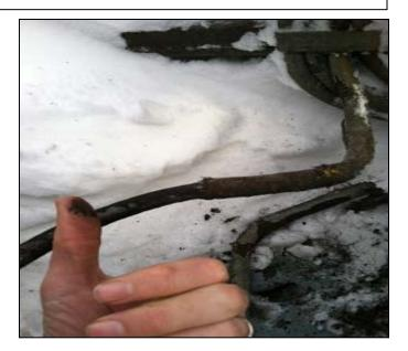
**Below:** (*Left*) Watertight integrity between SPAR deck and upper walking tunnel compromised. Wiring was being exposed to water and subsequently deteriorating over time. Wiring group from distribution panel passes through sheet metal penetration to overhead wire way. (*Right*) Chafing can cause excessive wear to sheathing and insulator and ultimately failure of the wire.
